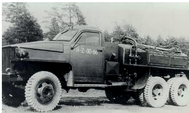
Рисунок 13 – Авторазливочная станция АРС-10, 1944 г. (фотография из архива 33 ЦНИИИ МО РФ) Figure 13: Chemical-spraying truck APC-10, 1944 (the photo is taken from the archives of the 33 Central Scientific Research Test Institute of the Ministry of Defence of the Russian Federation)
