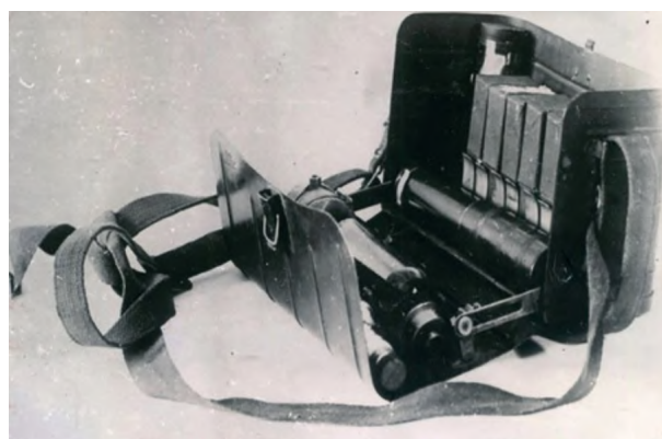
Рисунок 14 – Прибор химической разведки ПХР-43 (фотография из архива 33 ЦНИИИ МО РФ) Figure 14: Chemical agent detector kit ПХР-43 (the photo is taken from the archives of the 33 Central Scientific Research Test Institute of the Ministry of Defence of the Russian Federation)
